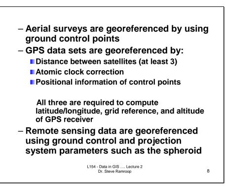
This slide shows the how aerial surveys, GPS, and Remote Sensing data are georeferenced. The role of ground control, and the mathematical formulae representation are major considerations.
